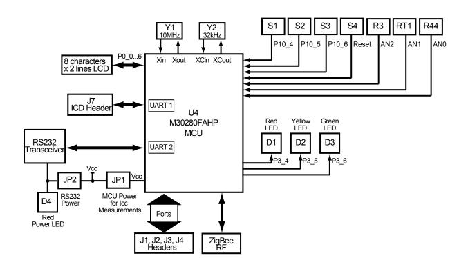
Figure 5-2: RZB-ZMD16C-ZDK Block Diagram
